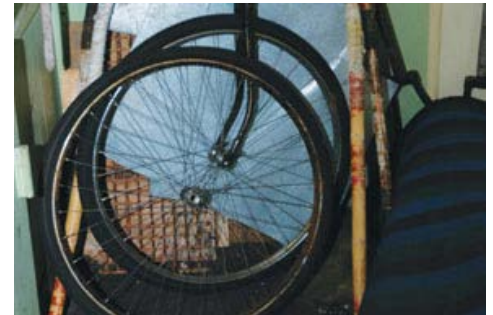
Bicycle wheels used to make sledge meters to measure the distance run
